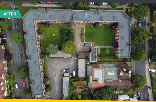
St Catherine's Court in Chiswick, West London provided a complex roofing challenge consisting of a deteriorating asphalt roof overlying a non-insulated concrete deck.
